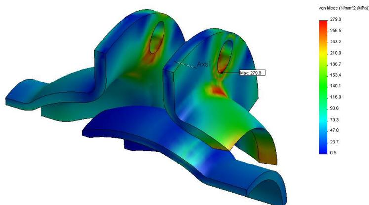
Fig. 8. Stress behaviour  $\sigma_{eff}$  at the pressure 4 MPa, armature DN50 – 4 bolts
