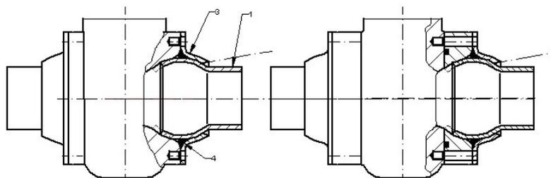
Fig.3 Solution alternatives of a armature connecting by means of the new flange joint
