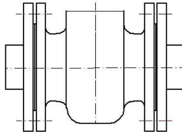
Fig.2 Common flange joint of an armature and a pipeline
