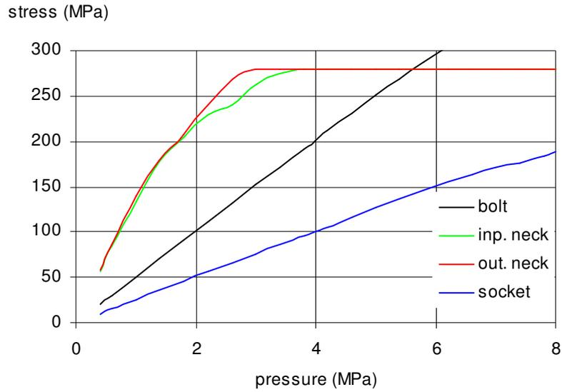
Fig. 9. Dependence of the component stress on the loading, armature DN50 – 4 bolts
