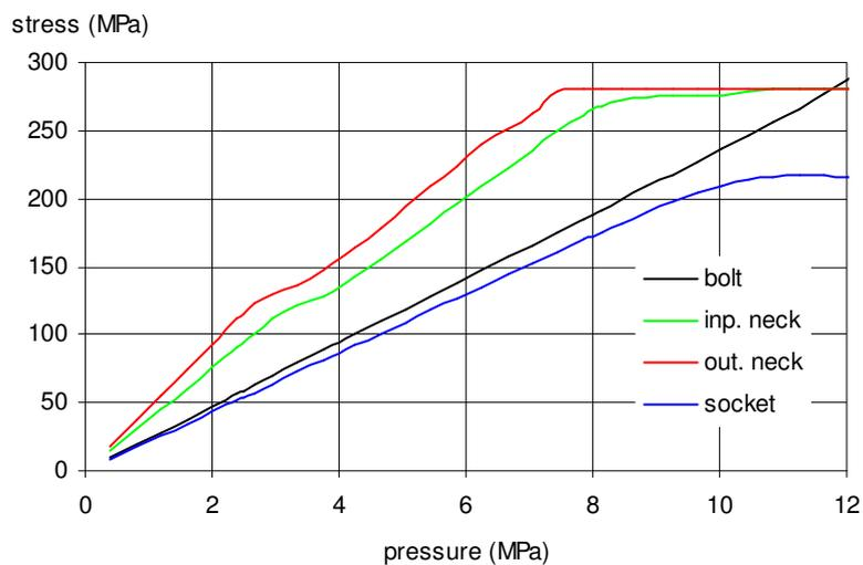
Fig. 11. Dependence of the component stress on the loading, armature DN50 – 8 bolts
