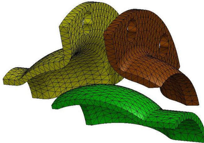
Fig. 4. Mesh model of finite elements for the joint DN50 – 8 bolts
