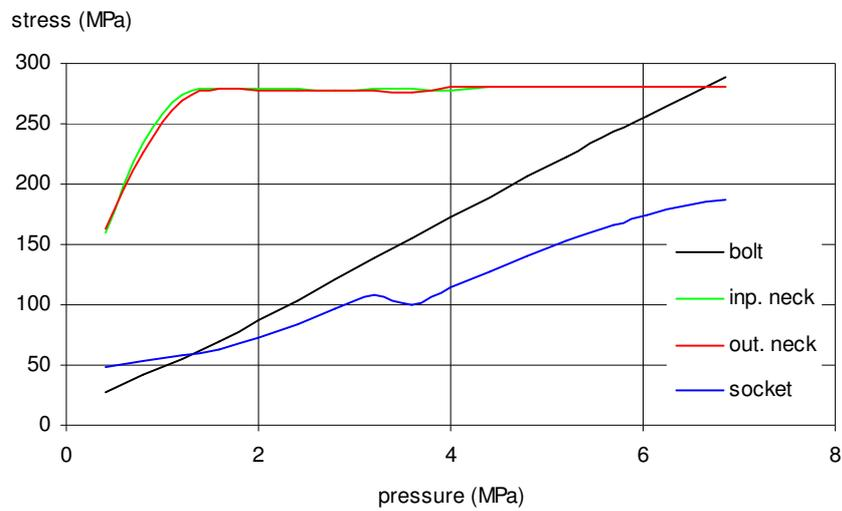
Fig. 13. Dependence of the component stress on the loading, armature DN125 – 4 bolts
