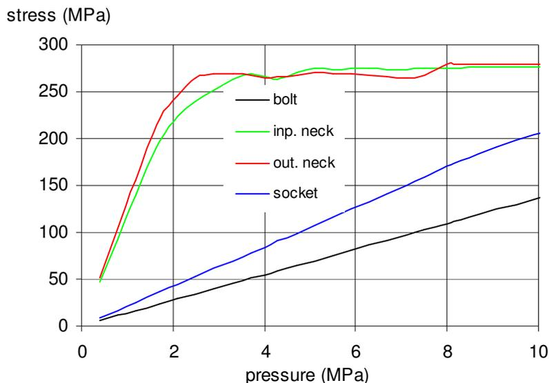
Fig. 15. Dependence of the component stress on the loading, armature DN125 – 8 bolts
