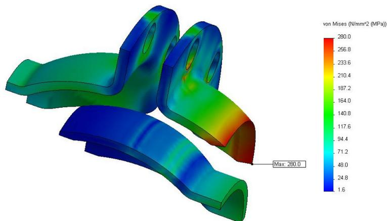
Fig. 14. Stress behaviour  $\sigma_{eff}$  at the pressure 8 MPa, armature DN125 – 8 bolts
