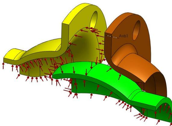
Fig. 6. Representation of model loading with internal overpressure
