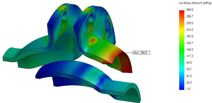
Fig. 10. Stress behaviour  $\sigma_{eff}$  at the pressure 8 MPa, armature DN50 – 8 bolts
