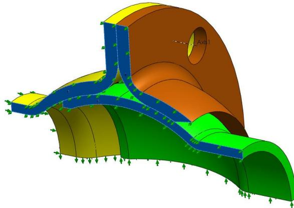
Fig. 5. Relation representation on the limits of symmetry and in an axial direction of the flange joint
