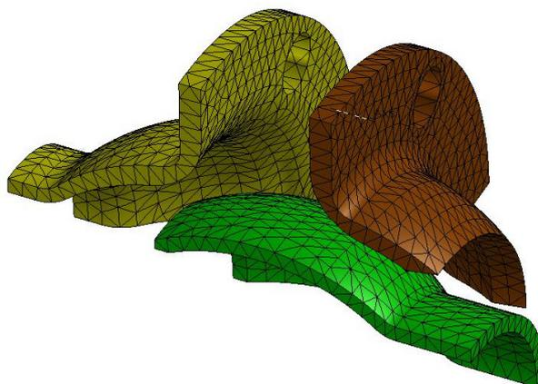
Fig. 3. Mesh model of finite elements for the joint DN50 – 4 bolts
