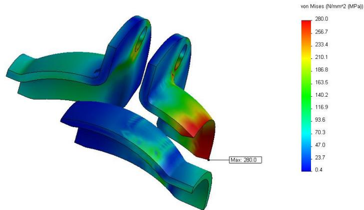
Fig. 12. Stress behaviour  $\sigma_{eff}$  at the pressure 6 MPa, armature DN125 – 4 bolts
